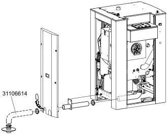
Remove the casings from the washer for easy access to the drain valve.
