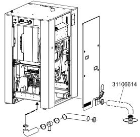
Remove the casings from the washer for easy access to the drain valve.
