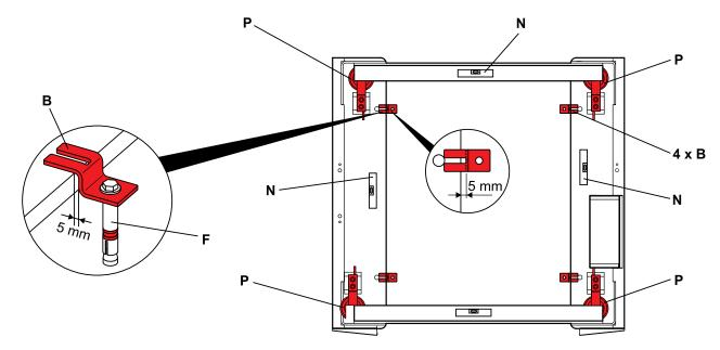
Weighing equipment: P Water level: N Fixing dowels: F Flange safety locks: B
