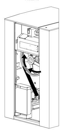
· Check the direction of rotation of the circulating pump and of the draught accelerator gas heating.
