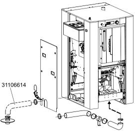
Remove the casings from the washer for easy access to the drain valve.
