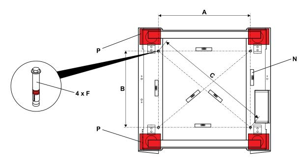
Mark out the drill holes for the securing dowels and drill them so as to insert the 4 dowels, they will secure the machine to the floor.
