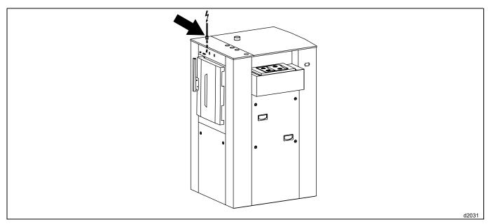
For each machine, install a fixed multipolar circuit breaker (or fuses protector) in the laundry main cabinet.
