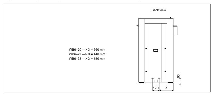
16.3 Drain connection at the left of the machine All washers
