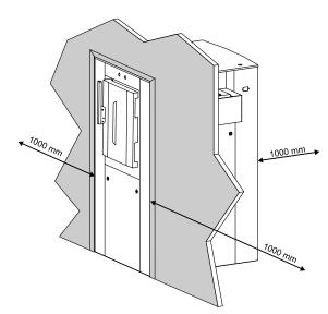
Leave at least 1 m (40") (according to the recommendation in standard EN 60204) between the machine, a wall or any other machine at the sides.
